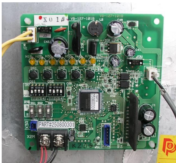
Figure 4, DIII-NET Communication Gateway mounted in unit
